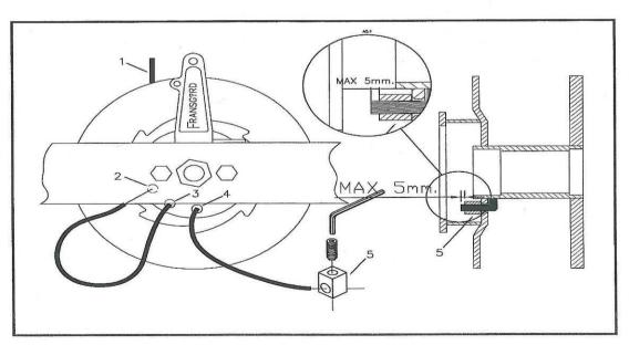
Drawing "B" Attaching cable to wire drum
